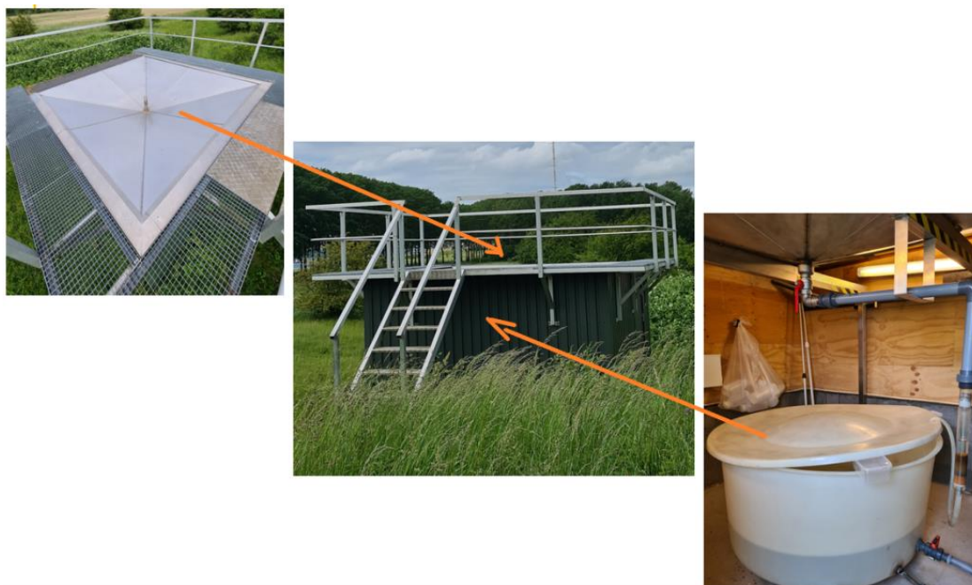
Figure 21: Rainwater collector. Shown on the top and inside of the housing where the water is collected into the large container
