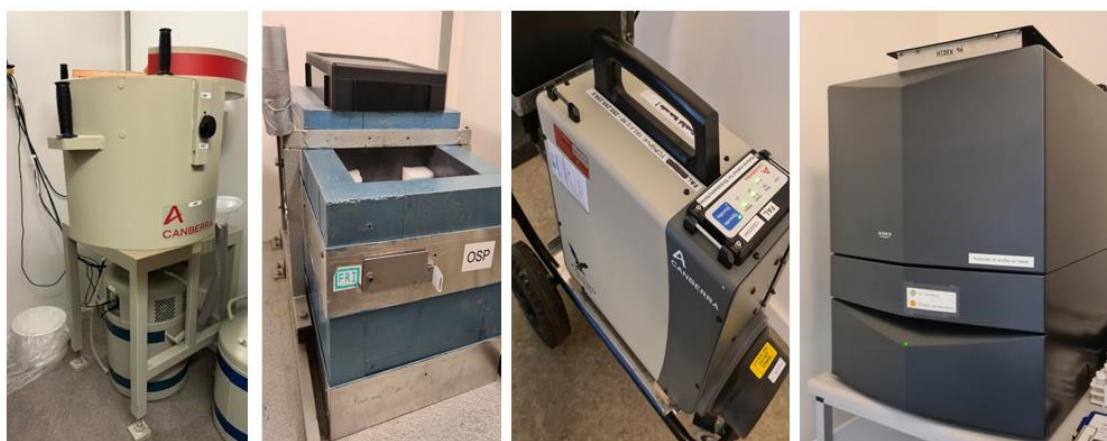
Figure 18: Counting equipment at the DHA/RP radionuclide identification and quantification laboratory (Mirion HPGe-detector, NaI-detector, portable Mirion HPGe-detector and Liquid scintillation counter-Hidex 300SL)
