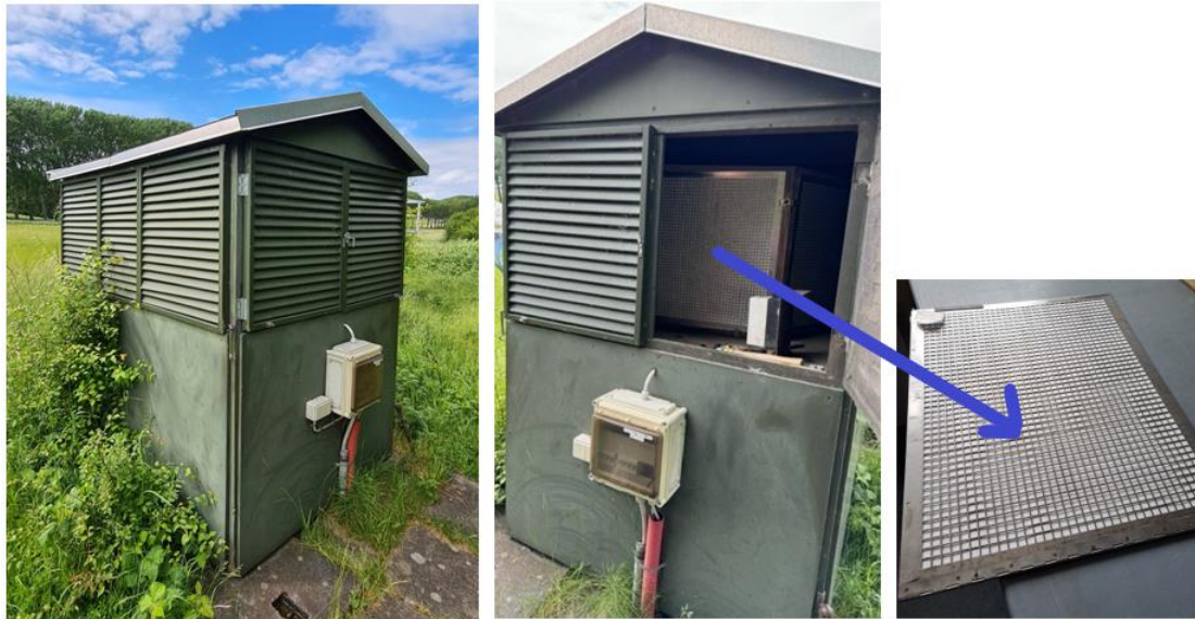
Figure 20: High volume air sampler at the DTU Risø Campus
