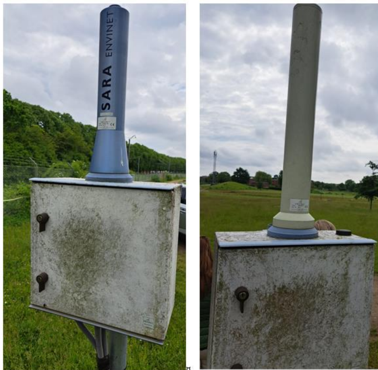
Figure 22: Automatic monitoring stations (Envinet SARA and GM)
