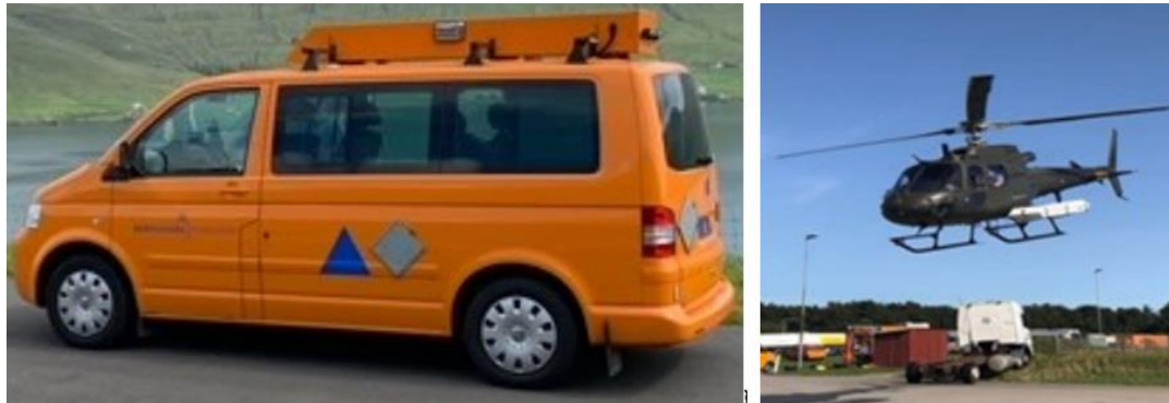
Figure 17: Car-borne and air-borne gamma spectrometry systems
