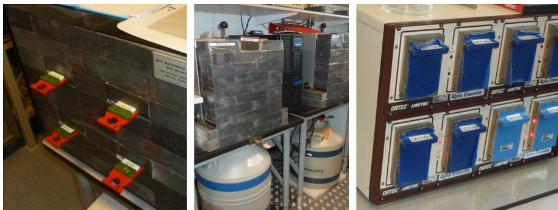
Figure 19: low level beta counter, gamma-spectrometers, alpha spectrometer at the DTU Sustain/RTS
