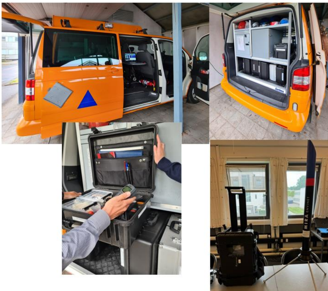
Figure 23: Car-borne gamma ray spectrometry system installed in a Volkswagen multivan, MIRA mobile autonomous dose rate monitoring station, MONA mobile spectroscopic detection and dose rate survey system
